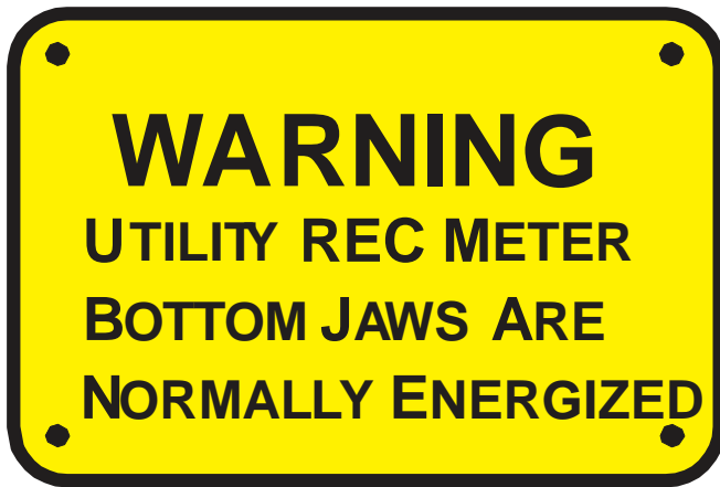
Tag 1: Install on Meter Box
